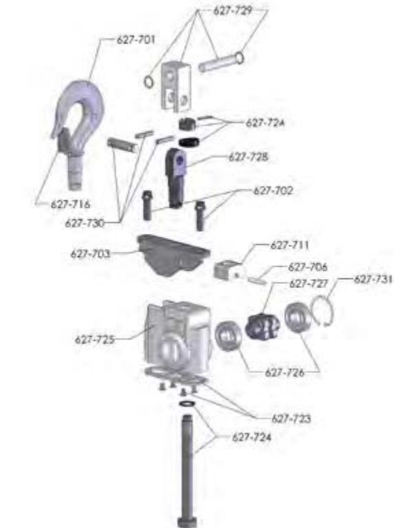
TRIPLE REEVED SUSPENSION & SHEAVE HANGER
